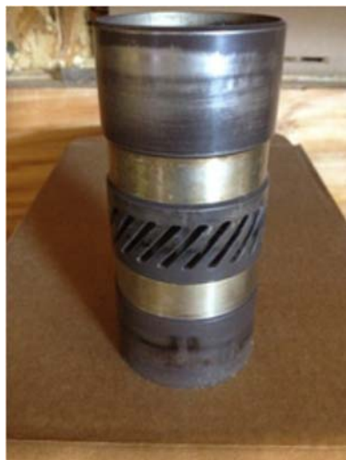
Figure 1: Spool Piece Wear
