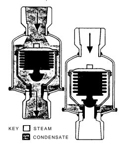
A true balanced pressure bellows is charged with water so that it follows the steam saturation curve very closely. (Some allowance is made for the spring rate of the bellows.) Twenty degrees below saturation temperature is typical. In case of a leak in the bellows, the tendency is to fail closed.
