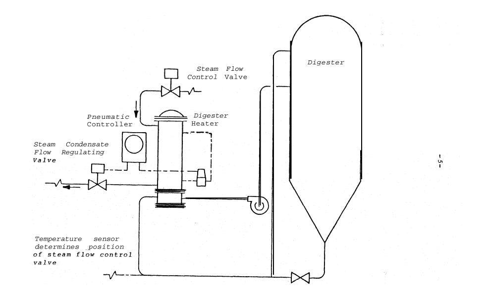
STEAM CONDENSATE DRAINAGE by MEANS of LEVEL CONTROL INSTRUMENTATION
