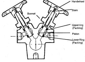
PTFE washer does soften as temperature rises. The softening helps the washer take the shape of the body and piston to assist sealing. The teflon helps lubricate the piston. Since the piston never clears the upper seals when open, the upper seals don't require metal reinforcement, and the softened PTFE is captured.
