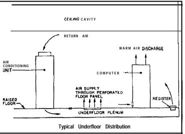
self contained with compressors or pumps, cooling coils and control systems, all mounted in an upright cabinet.
