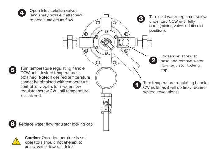
Note: To lock temperature and prevent adjustment, remove temperature regulating handle and install tamper resistant locking set (P/N D14924).
