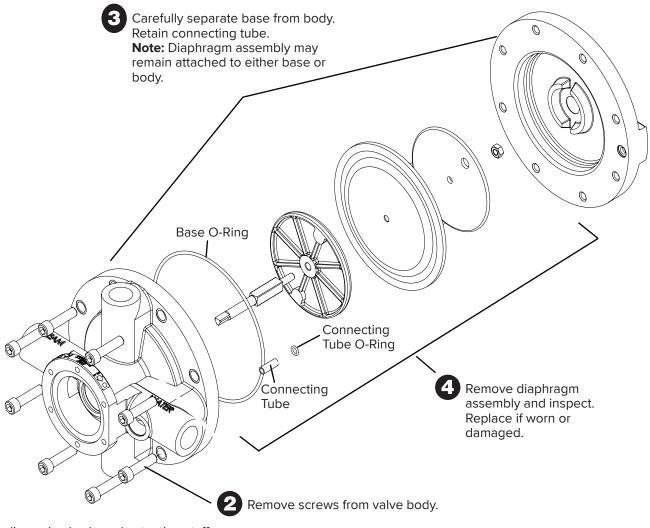
De-scaling valve body and actuating staff is recommended. Do not allow de-scaler to contact diaphragm if reusing it.
