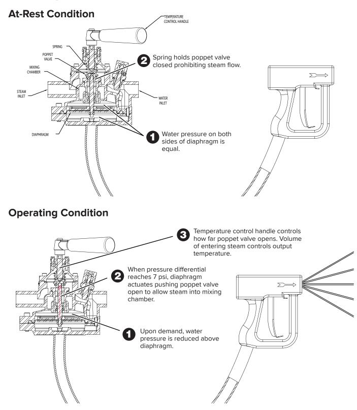
When demand ceases, equalizing water pressure reseats diaphragm in base of valve and spring closes poppet valve stopping steam flow.
