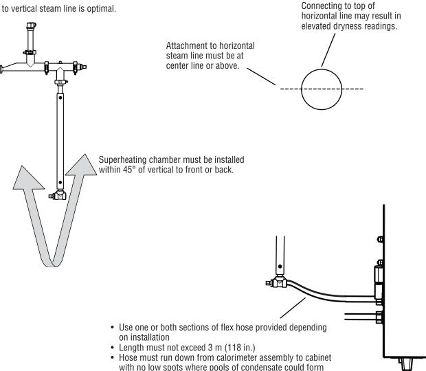
**Note**: Where necessary outlet on heating chamber can be rotated 180° to accommodate left or right cabinet position. See instructions below (p. 11).
