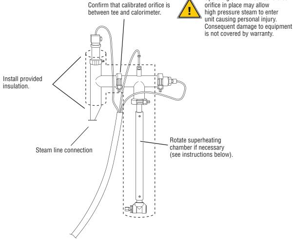
Rotate superheating chamber if necessary.
