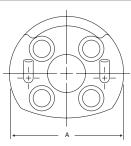
Valve seat retainer with guide pins, No. 5133-G, 5155-G, 6155-G traps.
