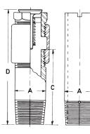
Tube with check valve and coupling.
