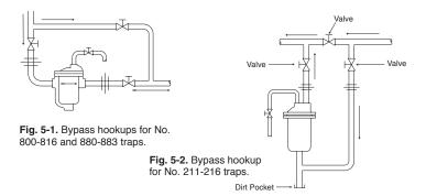
**Unions.** If only one is used, it should be on discharge side of trap. With two unions, avoid horizontal or vertical in-line installations. The best practice is to install at right angles as in Figs. 3-1 and 5-1 or parallel as in Fig. 5-2.
