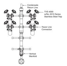
Fig. 4-1. Hookup for vertical manifold.
