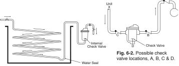
Fig. 6-1. Trap draining syphon.
