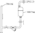
Fig. 4-2. Hookup for No. 1800 Series Stainless Steel trap.
