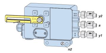
Following alignment and mounting of the positioner to the valve, pneumatic tubing has to be provided.
