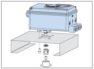
**Attention:** The feedback shaft **9** of the SRI has no mechanical stop, therefore may spin 360 degrees. The <u>permissible</u> rotation angle range is between +50 and -50 degrees around the arrow at the housing concerning the flat area of the feedback shaft (also see detail page 13 bottom). Since a rotary actuator has a rotary angle of about 90 degrees the mounting as described in the following must be carried out very precisely.
