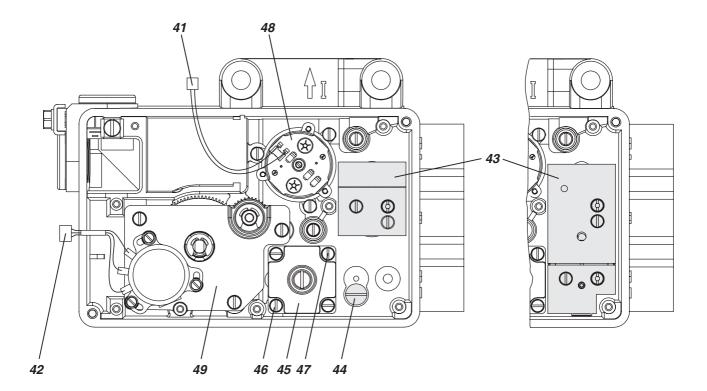
The base plate consists of a manifold and air ducts. O-rings are required to guarantee sealing of the mounted elements.
