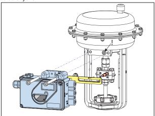
The attachment of the positioner is accomplished by bolting it directly to the actuator yoke using the feedback lever for a direct mount (with attachment kit EBZG -D).
