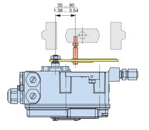
Carrier bolt for connection to valve stem
