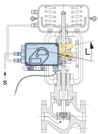
Direction of rotation of feedback shaft of a single-acting **stroke actuator** with spring:
