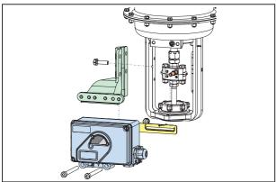
Attachment of the positioner to the actuator is made to the left using the mounting bracket and feedback lever for a NAMUR mount. Use:
