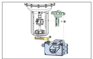
Attachment of the positioner to the actuator is made to the right using the mounting bracket and feedback lever for a NAMUR mount. Use:
