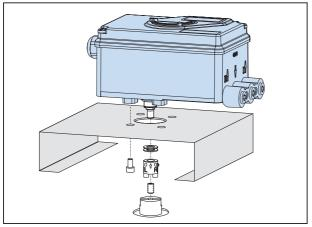
**Attention:** The feedback shaft *9* of the SRD has no mechanical stop, therefore may spin 360 degrees. The <u>permissible</u> rotation angle range is between +50 and -50 degrees around the arrow at the housing concerning the flat area of the feedback shaft (also see detail page 17 bottom). Since a rotary actuator has a rotary angle of about 90 degrees the mounting as described in the following must be carried out very precisely.
