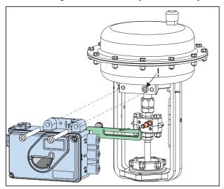
The attachment of the positioner is accomplished by bolting it directly to the actuator yoke using the feedback lever for a direct mount (with attachment kit EBZG -D).
