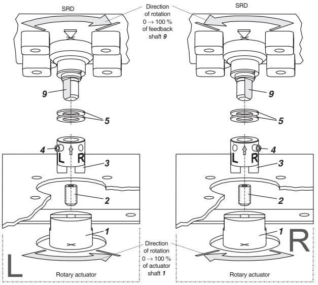
Figure 27: Mounting if actuator is left-rotating
