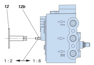
Turn the travel indicator 12 to the desired position, put it on the gear shaft against the stop and pinch the wire ring for secure coupling.
