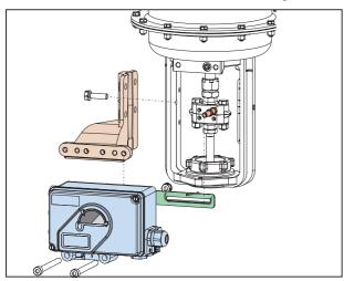
Attachment of the positioner to the actuator is made to the left using the mounting bracket and feedback lever for a NAMUR mount. Use:
