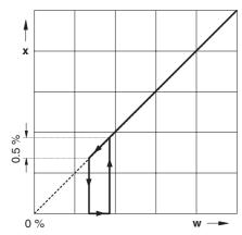
Sealing tightly, linear charcteristic line
