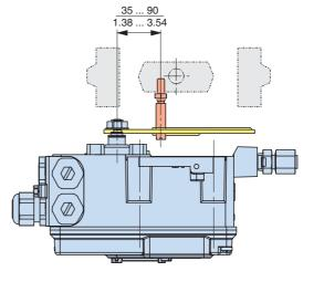
Carrier bolt for connection to valve stem
