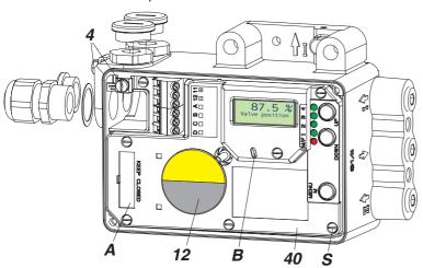
If the SRD is equipped with option "IrCom" **B**, communication can take place contactless via infrared with the positioner (even with closed cover!). Modem "IR Interface" (not Ex) is connected via RS232 to a PC (for practical reasons a notebook) with software PC20 / PC50 and makes possible a range of approx. 1 m.
