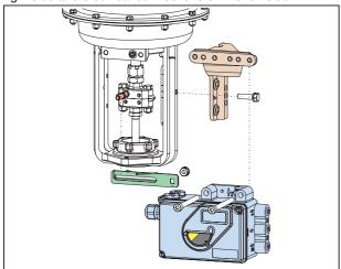
Attachment of the positioner to the actuator is made to the right using the mounting bracket and feedback lever for a NAMUR mount. Use:
