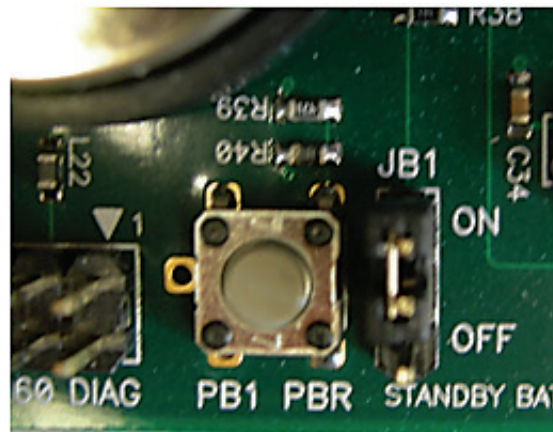
Figure 3-1. Standby Battery Jumper JB1
