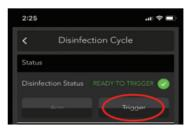
The message "Ready to Trigger" will appear once the product has acknowledged the request. Tap "Trigger" to confirm and initiate the disinfection cycle within 30 seconds of arming. Failure to trigger will require the Arm process to be repeated.
