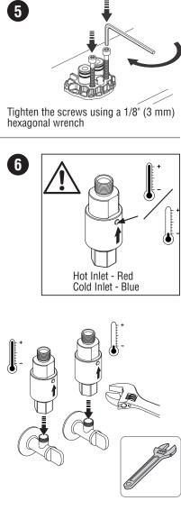
**DO NOT** use jointing paste when making plumbing connections.
