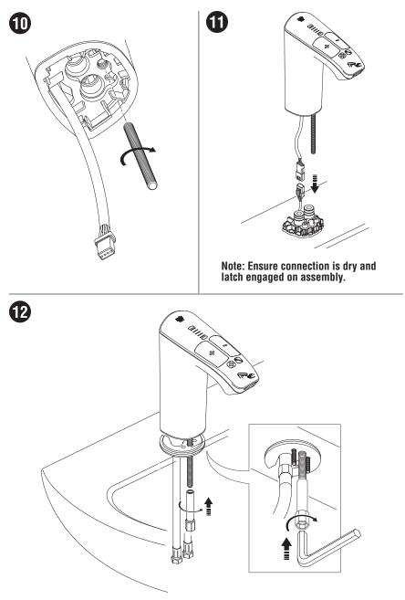
Tighten the nut using a 7/23" (6 mm) hexagonal wrench.
