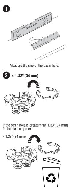
If the basin hole is smaller than 1.33" (34 mm) discard the plastic spacer.
