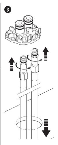
Install the flexible tails or rigid pipes.
