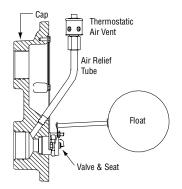
Figure 4. Float & Thermostatic Trap
