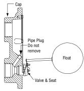
Figure 6. Liquid Drainer
