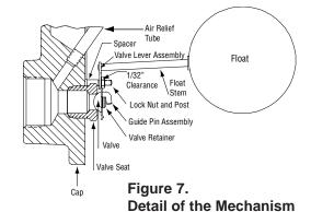
Note: Never replace only a valve or only a valve seat. Be sure that new valve and seat are the correct orifice size for your operating pressure. The orifice size is stamped on the valve seat, valve lever, and guide pin assembly.
