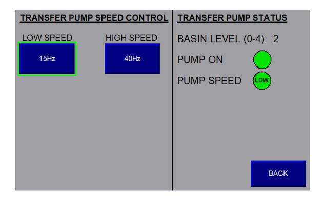
The water level in the lower basin is at the second float switch. The transfer pump is running at LOW speed.
