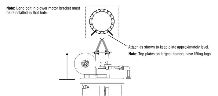
4. Remove top plate from lower canister.
