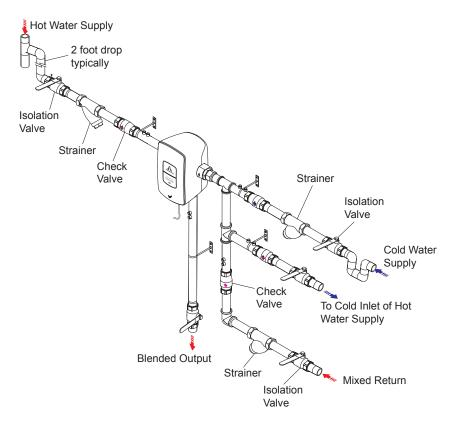
Make sure that each pipe is connected in the correct location in the system and in the proper orientation.
