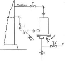
**Figure 1.** Installation of ball float drainer for medium or heavy loads. Strainer blow-down valve "B" and drainer blow-down valve "C" are optional. Discharge line valve "D" not required if drainer discharges water to ground.
