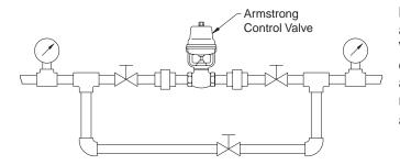
**Note:** The Armstrong ECV and ACV control valves are suitable for a variety of fluid control services. When installing the control valve be certain that the direction of flow conforms to the direction of the arrow stamped into the casting and that the maximum operating pressure (MOP) of the valve is adequate for the installation.
