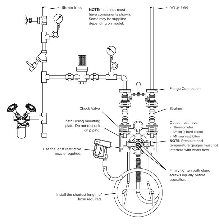
**Note:** Code or regulatory requirements may include back-flow preventers (single or double action) or vacuum breakers, which are not listed above.
