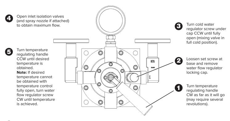
6 Replace water flow regulator locking cap.
