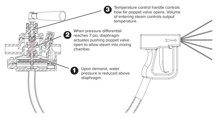
When demand ceases, equalizing water pressure reseats diaphragm in base of valve and spring closes poppet valve stopping steam flow.
