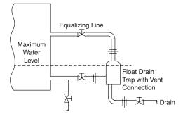
**Figure 3.** Liquid drainer trap installed at side of a receiver, close to floor. Water will rise to broken line before drain trap opens.
