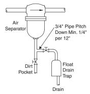
**Figure 2.** Installation of a liquid drain trap on side of separator.
