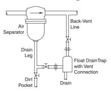
**Figure 1.** Installation of a liquid drainer with equalizing line downstream of the separator in order to assure a quick and regular flow to the drainer. Note side inlet connection from separator.
