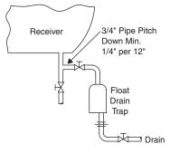
**Figure 4.** Install the drain trap on side to get better access or compensate for lack of space under the receiver (particularly for drain trap used under compressors).
