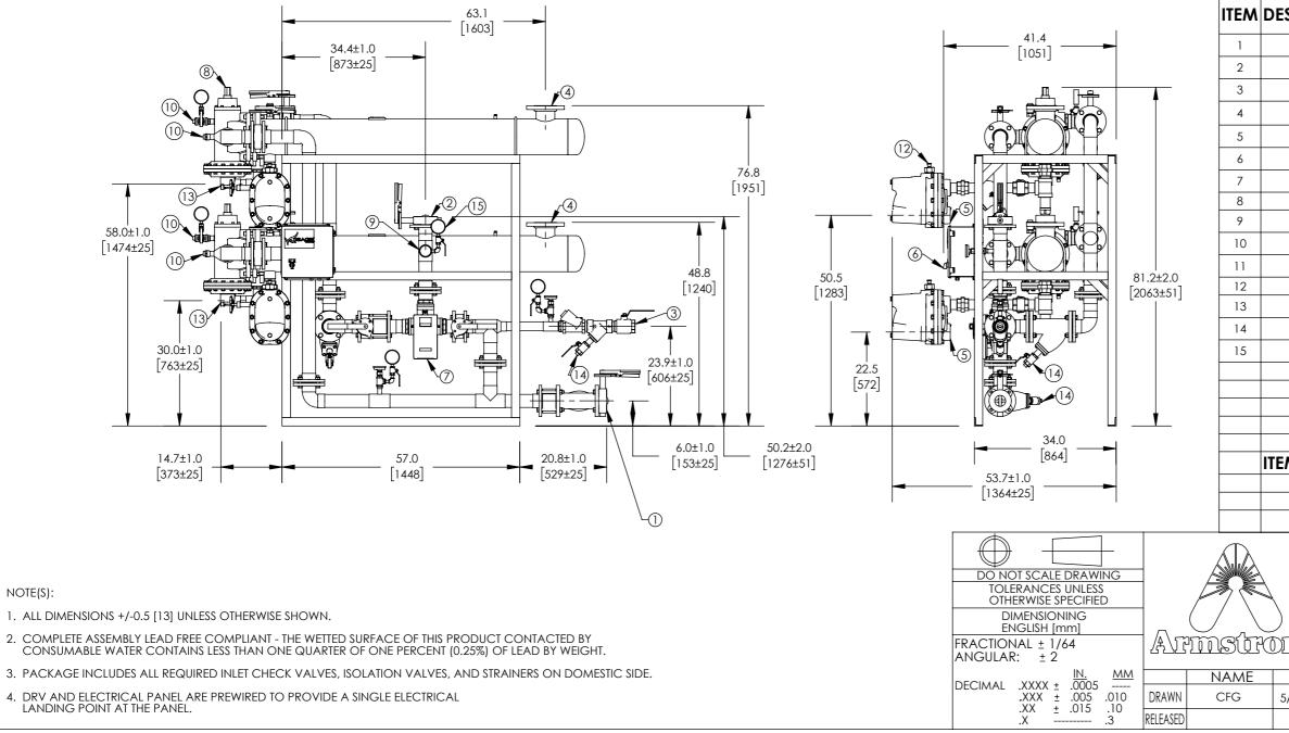
4. DRV AND ELECTRICAL PANEL ARE PREWIRED TO PROVIDE A SINGLE ELECTRICAL LANDING POINT AT THE PANEL.
