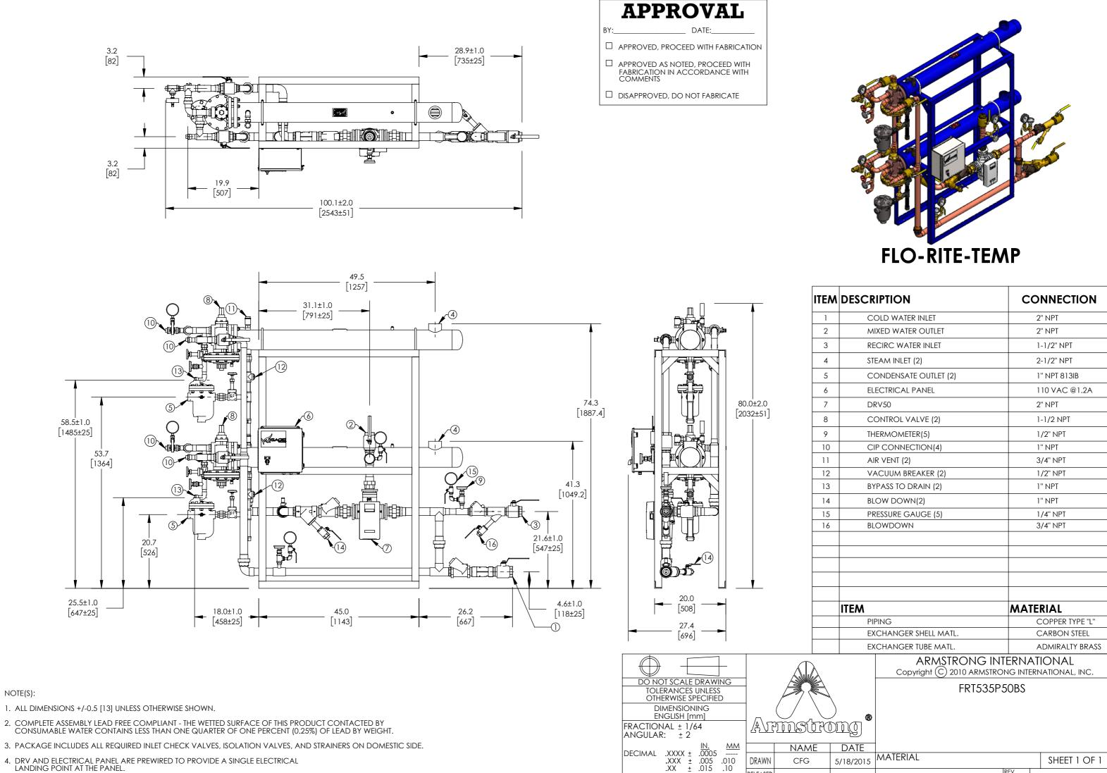
4. DRV AND ELECTRICAL PANEL ARE PREWIRED TO PROVIDE A SINGLE ELECTRICAL LANDING POINT AT THE PANEL.
