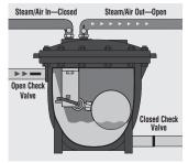
**Filling** 1. During filling, the steam, air or inert gas inlet and check valve on pumping trap outlet are closed. The vent and check valve on the inlet are open.
