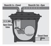
**Repeat Filling** 4. Steam, air or inert gas inlet and trap outlet are again closed while vent and condensate inlet are open. Cycle begins anew.
