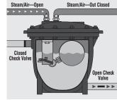
**Begin Pumping** 2. Float rises with level of condensate until it passes trip point, and then snap action reverses the internal valve positions shown in step one.
