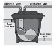
**End Pumping** 3. Float is lowered as level of condensate falls until snap action again reverses the internal valve positions.
