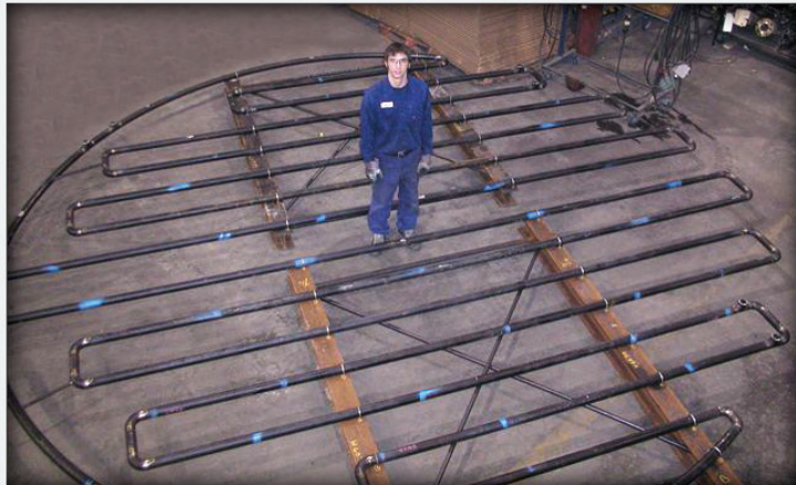
Full Tank Area Tank Heater
