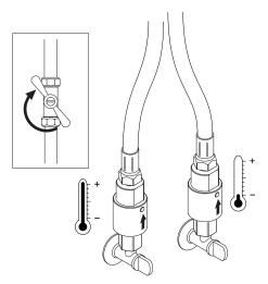
Open hot and cold water supply and check for leaks.
