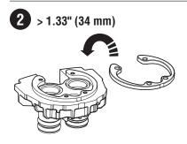
If the basin hole is greater than 1.33" (34 mm) fit the plastic spacer.
