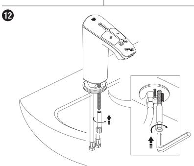
Tighten the nut using a 7/23" (6 mm) hexagonal wrench.
