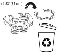
If the basin hole is smaller than 1.33" (34 mm) discard the plastic spacer.
