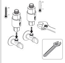
**DO NOT** use jointing paste when making plumbing connections.
