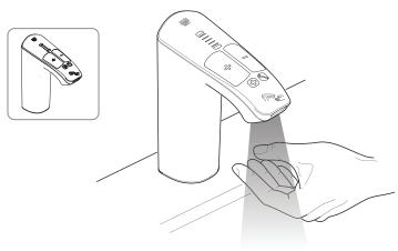
To increase the water temperature place your hand above or next to the Red + Indicator. It is not necessary to make physical contact with the faucet itself.
