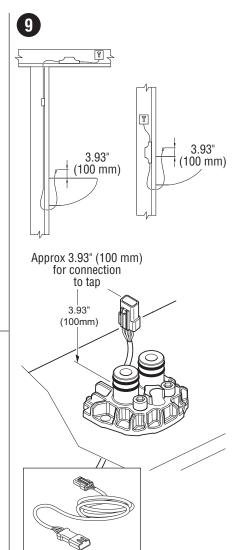
Note: Make sure that you install the PSU (Power Supply Unit) in an area that you can access easily for servicing and maintenance purposes. Ensure connection to tap is dry and latch engaged on assembly.
