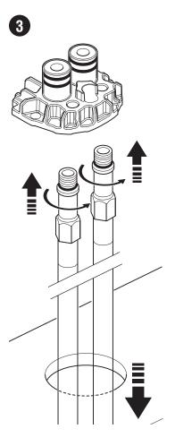
Install the flexible tails or rigid pipes.
