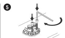
Tighten the screws using a 1/8" (3 mm) hexagonal wrench
